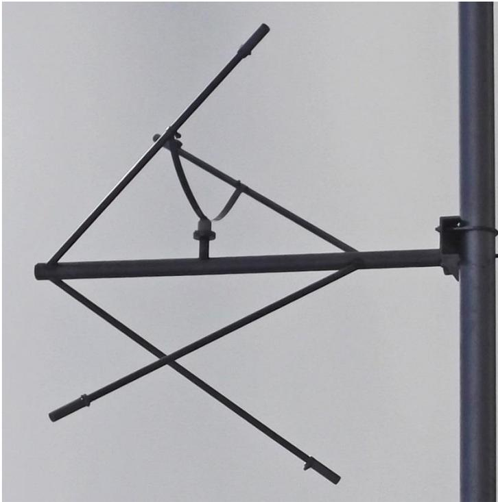
A single bay **FMP** is fed directly, while multi-bays are fed with a power divider. Input power ranges from 3 kW with a single bay to 24 kW with an 8-bay antenna. The maximum ERP of the **FMP** is 1.47 kW with a single bay and 60 kW with an 8 bay antenna. Since the multi-bay **FMP** antennas are branch fed, there is no differential group delay across the channel, making this a perfect choice for ATSC 1.0 and 3.0 operations
